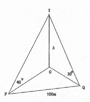
A surveyor stands at a point P due south of a tower OT of height h, and finds the angle of elevation of the top of the tower to be  $40^{\circ}$ . And then walks 100m to a point Q, so that the angle POQ is  $90^{\circ}$ , and finds that the angle of elevation from Q is  $30^{\circ}$
